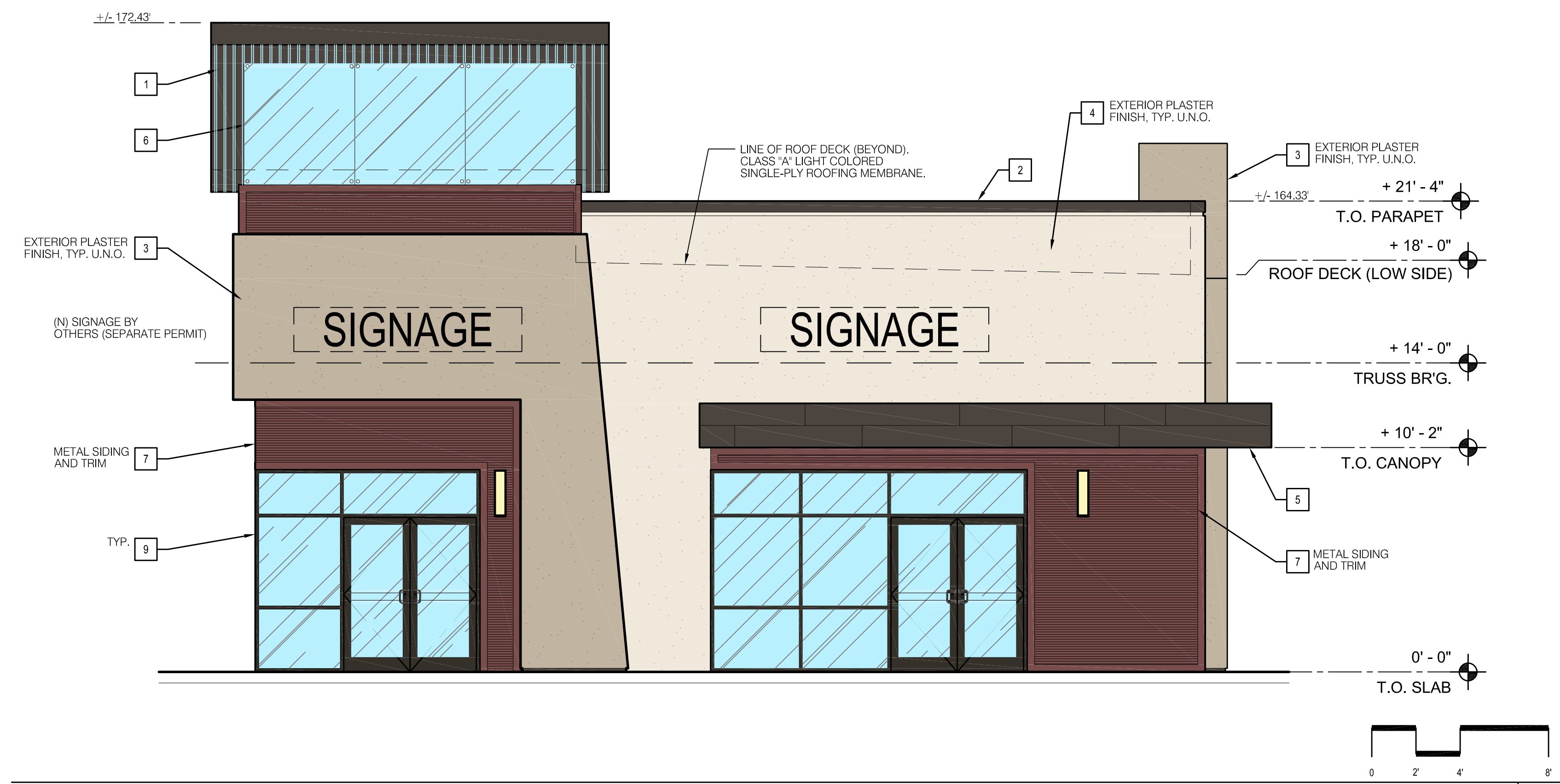
PROPOSED EAST ELEVATION 1/4" = 1'-0" B
