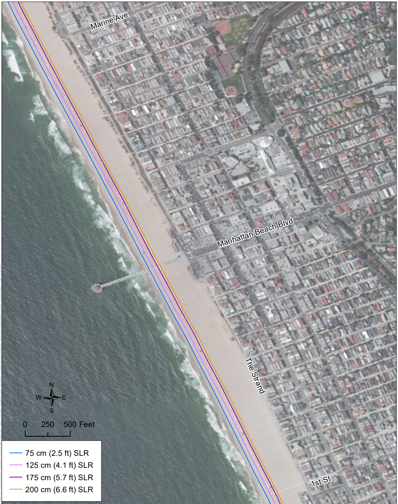
Figure 3-10 Shoreline Erosion with Sea Level Rise in South Manhattan Beach
