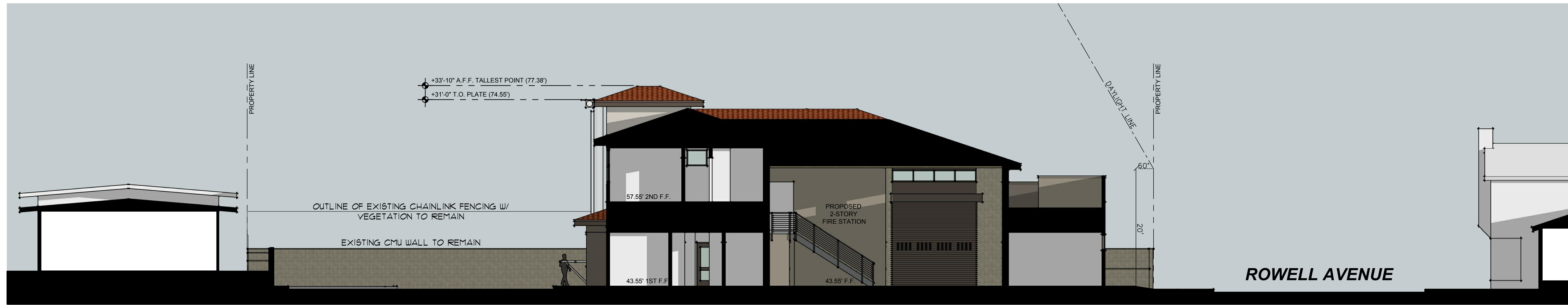
SECTION VIEW A: EAST-WEST SECTION THROUGH APPARATUS BAY
