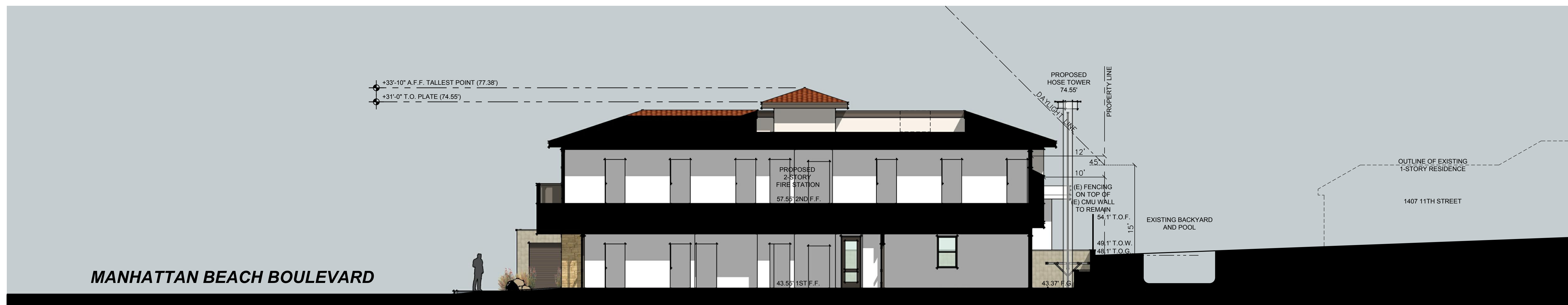
SECTION VIEW C: NORTH-SOUTH SECTION THROUGH FIRE STATION
