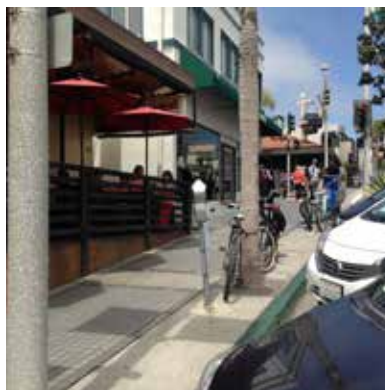
-F2 Bike parking that uses light poles, palm trees and meters, conflict with the width of the walkway and hinder pedestrian movement
