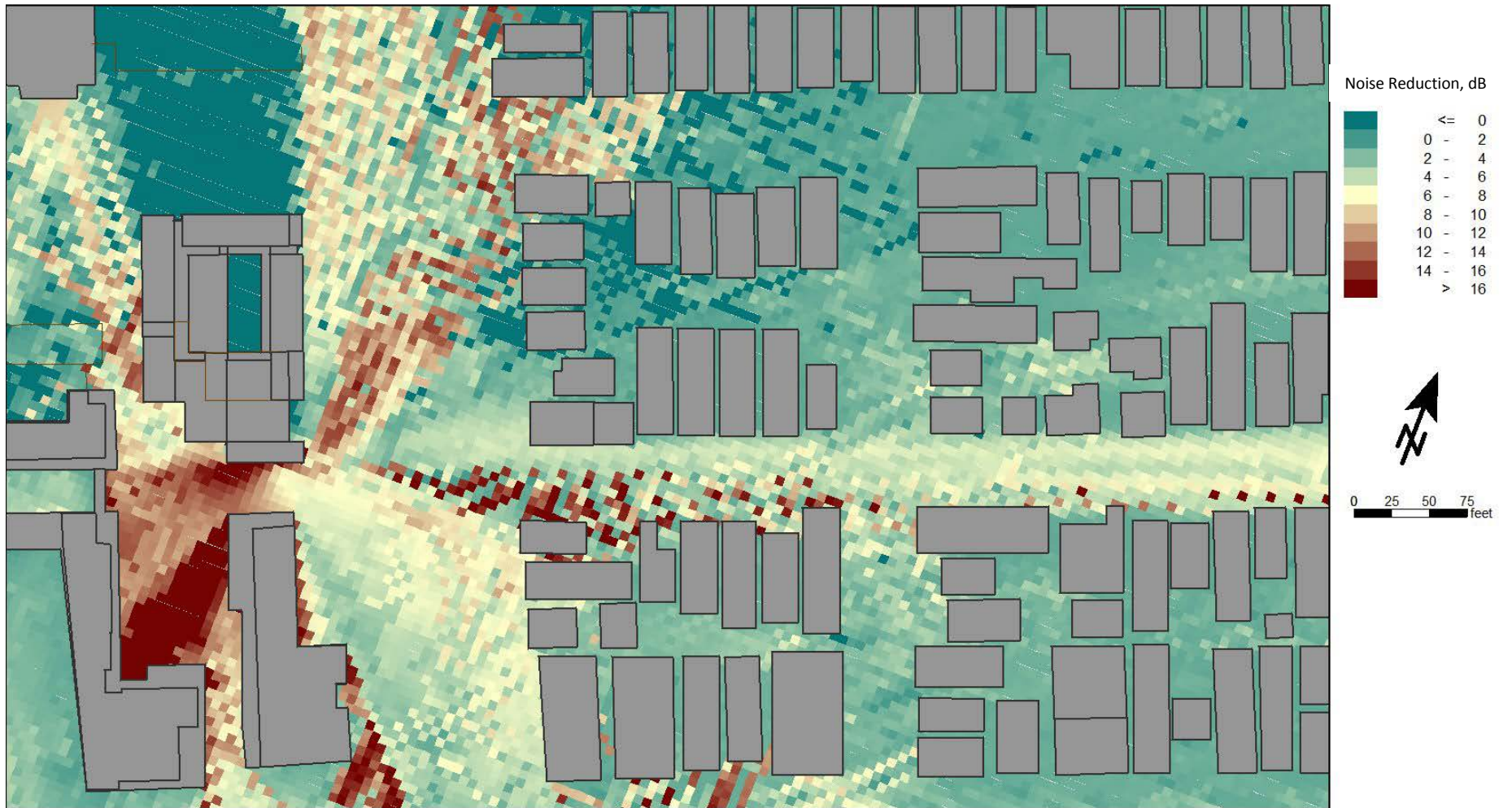
Figure 3. Mitigated South Terrace Difference Map at 1 st Floor with Sound Rated Curtains (Scenario 1)
