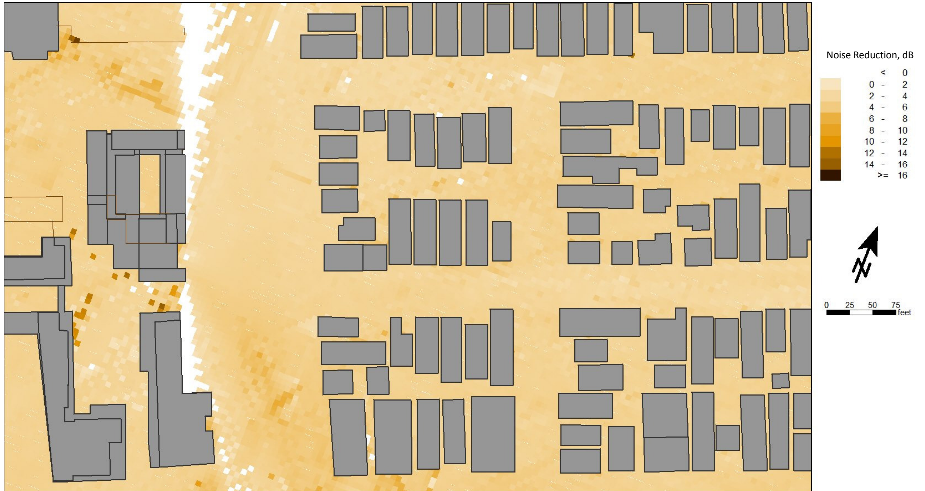
Figure 3. Noise Difference Map - Reduction of Front Entrance Noise at 1 st Floor
