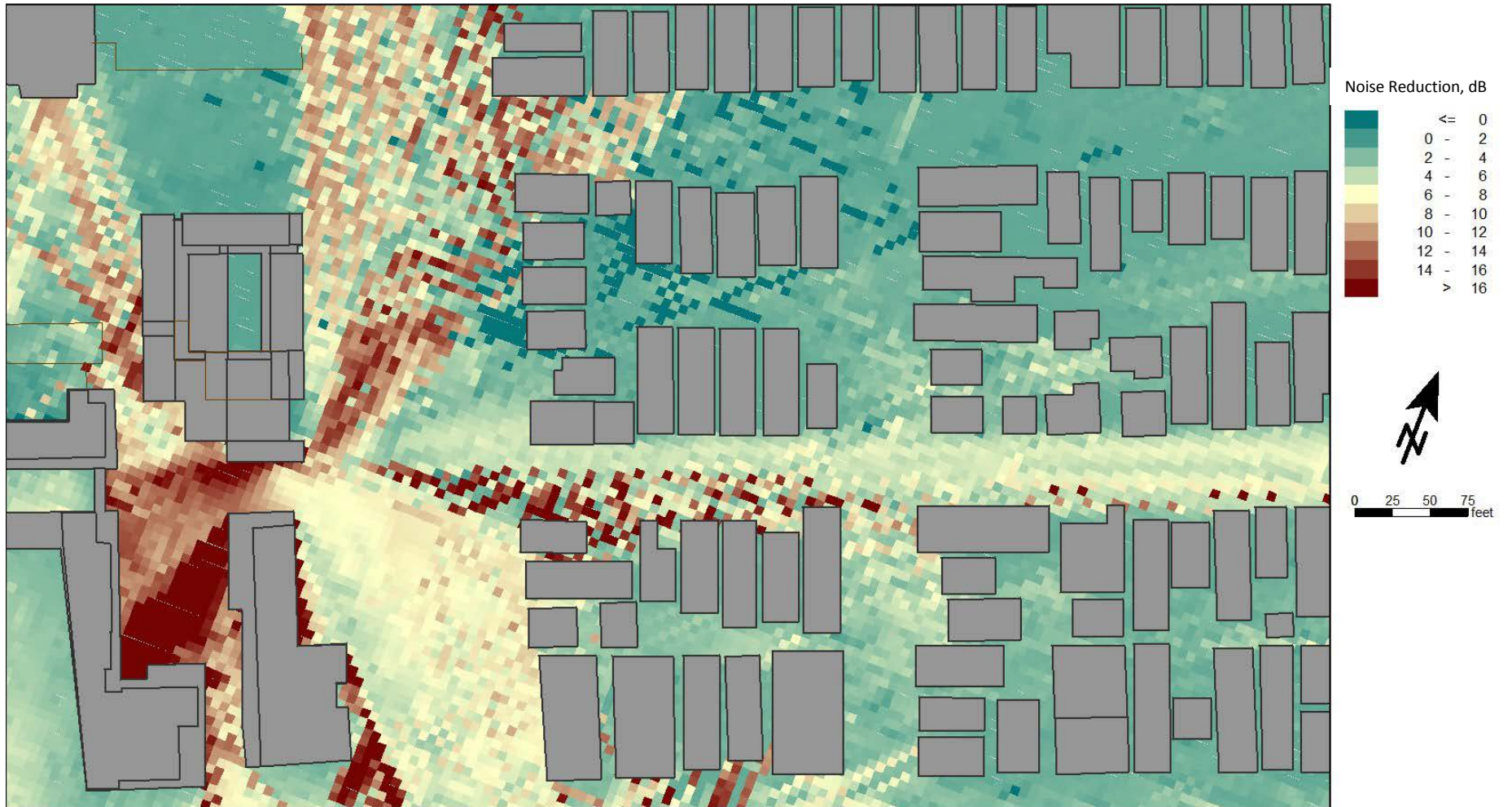
Figure 7. Mitigated South Terrace Difference Map at 1 st Floor with Sound Rated Curtains, Awning and Petros Living Wall (Scenario 3)
