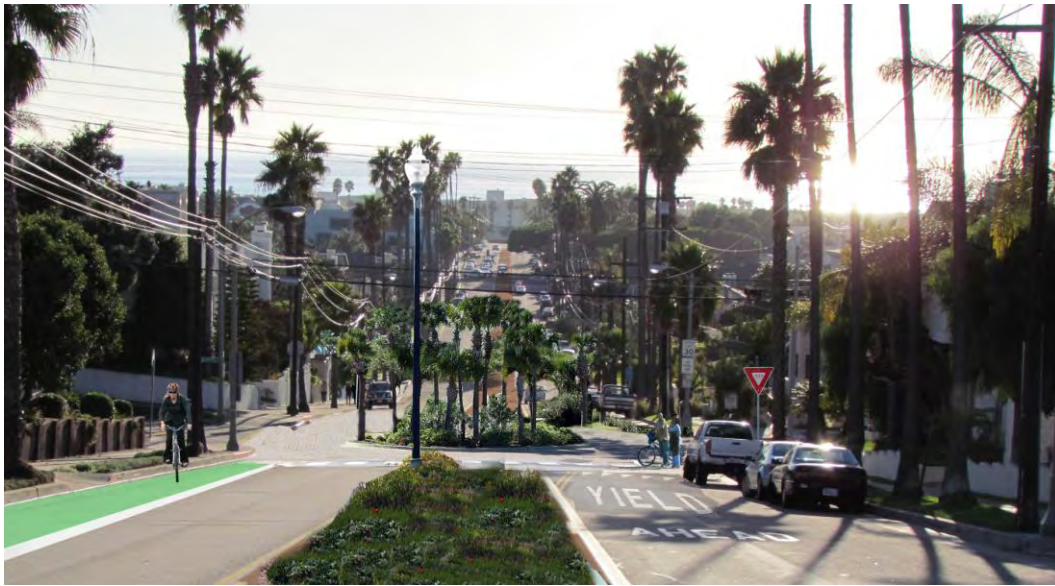
Add bike lanes in accordance with the South Bay Bicycle Master Plan. Often, bicyclists need "climbing lanes" on hilly roads. This photo-visualization shows a climbing lane and a traffic circle added to Beryl St.
