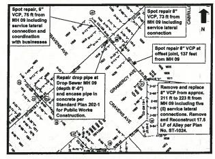
CBM is providing Construction Observation for the City of Torrance performing citywide spot repairs and cleaning. The Project includes video-inspector, point repairs, removal and replacement, pipe-lining, manholes; alley reconstruction, curb and gutter, sidewalk reconstruction and traffic control.
