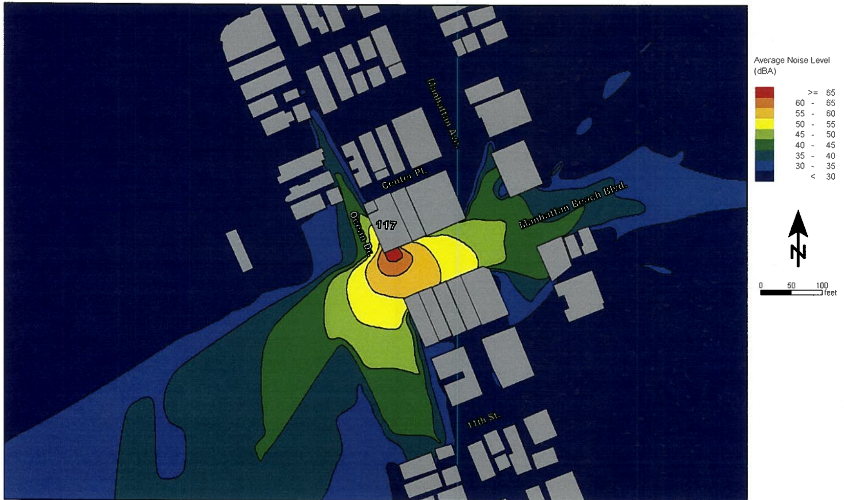
Figure 3. Modeled Average Noise Level of Proposed Strata Project at 1 st Floor with Windows Closed and Patios and Balconies Occupied
