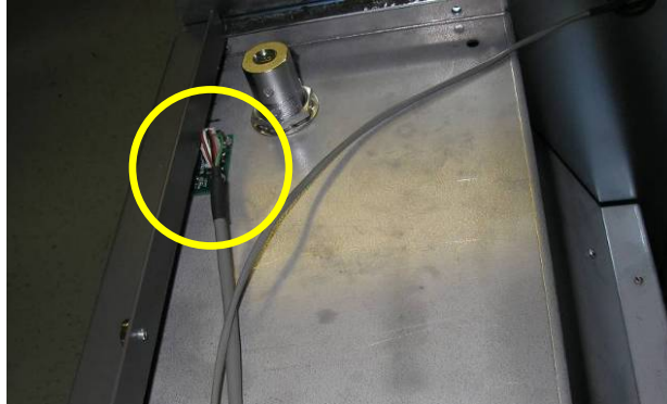
Figure 29. Top view: Front door sensor
