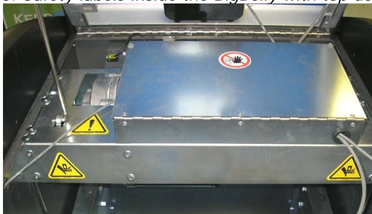
Figure 3. Safety labels inside the BigBelly with top door open
