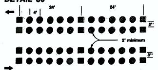
Alternate to Detail 29. For use at problem locations where it is difficult to place and maintain lines because of moisture, sand, etc.
