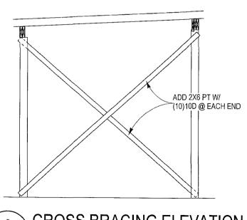
2 CROSS BRACING ELEVATION S1 SCALE: 1/4" = 1'-0"
