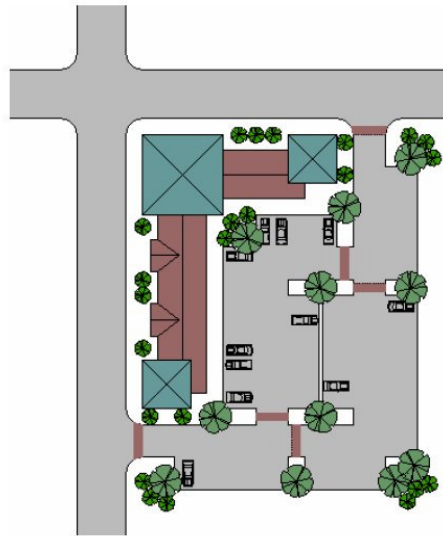
Figure 13: Example of Corner Buildings With Parking In the Rear
